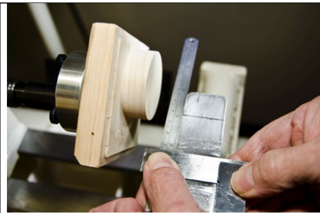
Figure 16 – Using a ruler to position the small square at a precise distance from the center turning axis mark on the tool rest
