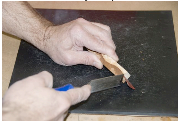
Pic 8: Trim off excess glue and veneer with a sharp chisel
