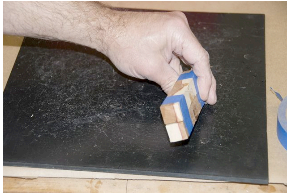
Pic 10: Blanks restacked and taped for the 2 nd cut
