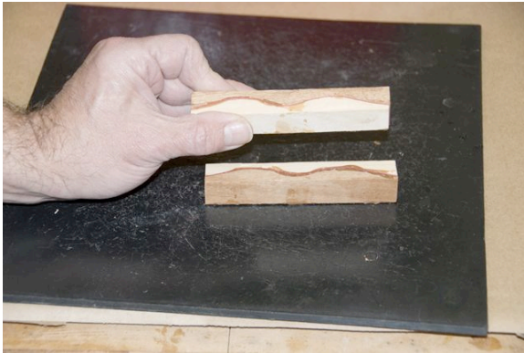
Pic 9: Restacking blanks, aligning the previous cut line
