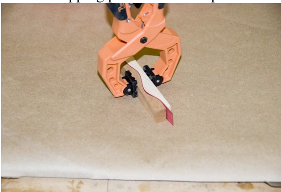
Pic 5: Temporary clamp keep parts aligned
