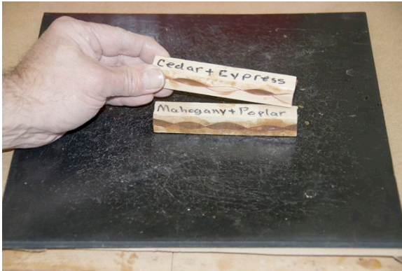
Pic 13: Swapping blanks between pairs gets 2 blanks containing all 4 woods
