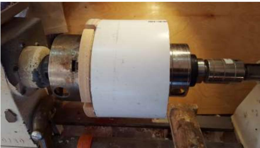
The picture below shows the live center adapter and Talon chuck for this operation.
