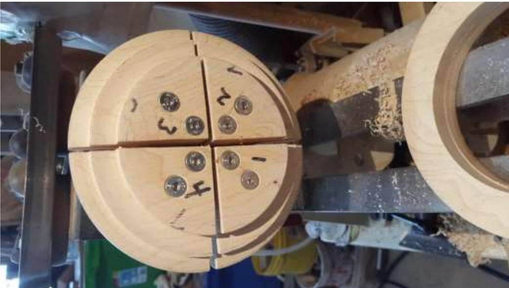
Place the top onto the step jaws.
