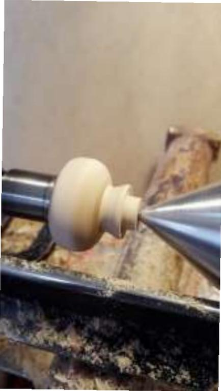
Use a Step type center drive and form the 1/2" inch or 9/16 inch tenon at the tailstock end. Sand the knob as needed for a good smooth finish.
