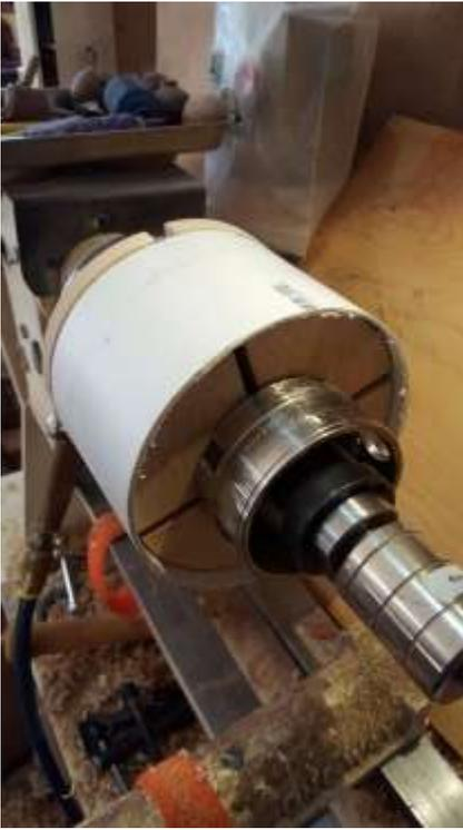
Turn on the lathe, about medium speed and carefully true up the end of the PVC pipe at the tailstock end. Stop the lathe, loosen up both chucks, turn the PVC around, tighten both chucks and again true up the PVC at the tailstock end. I use the Hunter #1 tool, see the picture below.
