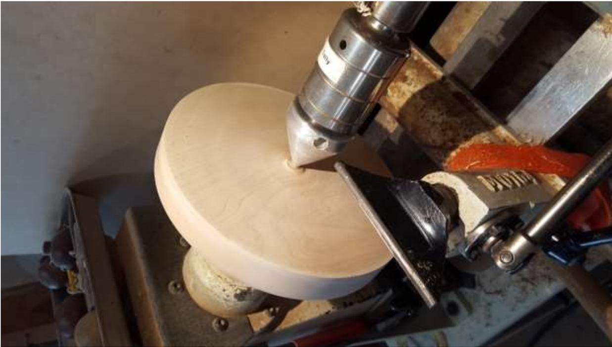
Using a compass, or dividers, mark a circle about 6 to 6 $\frac{1}{8}$ ". Remember to allow for fabric on the PVC, test the fit with the fabric glued onto the PVC. The groove can be from  $\frac{1}{8}$ " to  $\frac{1}{4}$ " deep depending on the thickness of the wood used. You will get a feel for this step as you progress along.
