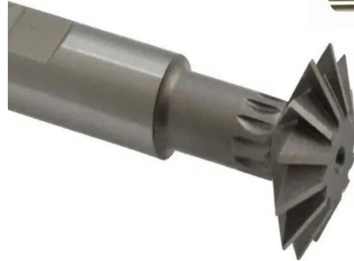
3/4x3/16, 10 tooth, HSS 60 degree double angle cutter 3/8 th Shank
